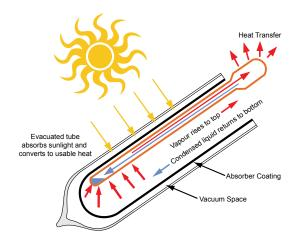
**Step 1.** The sunlight strikes the dark absorber coating inside the evacuated tube.
